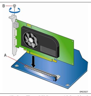
Figure 17. Installing a PCI Express x16 Graphics Card
